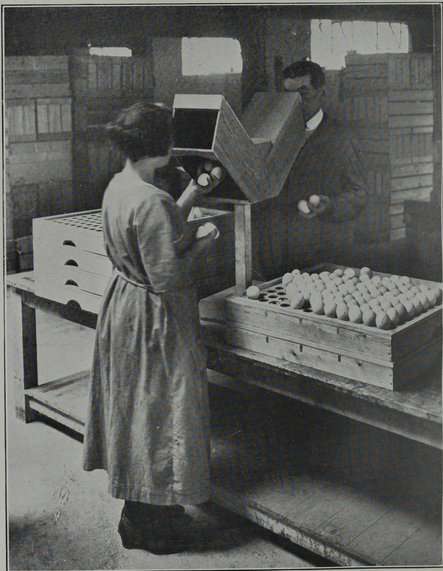
FIG. 6.—“Daylight Tester,” i.e. , apparatus fitted with electric light and shutters to obviate necessity for a dark room.
